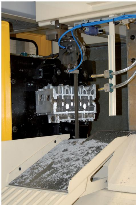
For more than 20 years, Siif has designed and manufactured band saws for cutting aluminum risers and feeders.
