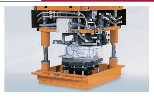
Siif provides trimming dies for aluminum castings produced in high pressure die casting, low pressure or gravity die casting.
