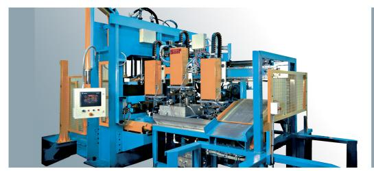
By integrating the best measuring and non-destructive test equipment, SiiF carries out the inspection operations specified by the manufacturer downstream of the finishing process.
