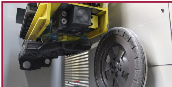
Snag grinding with diamond coated wheel
