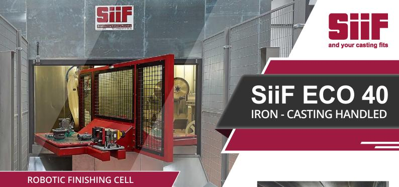
Casting max. dimensions 500 mm x 500 mm x 400 mm Casting max. weight 40 kg
