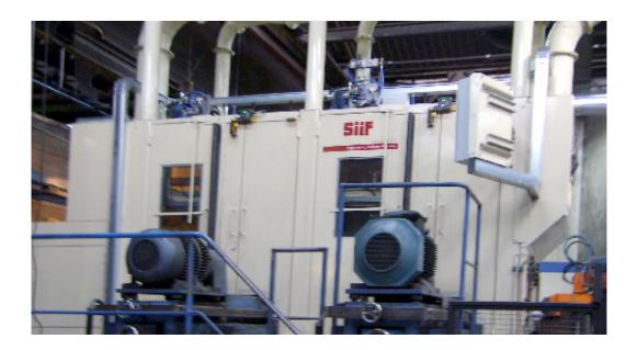
For the finishing of iron engine blocks and cylinder heads SiiF proposes 4 faces grinding machines.
