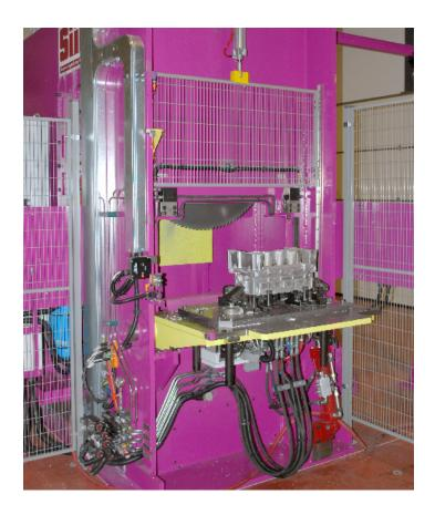
SiiF has developed a circular saw for cutting aluminum risers and feeders.
