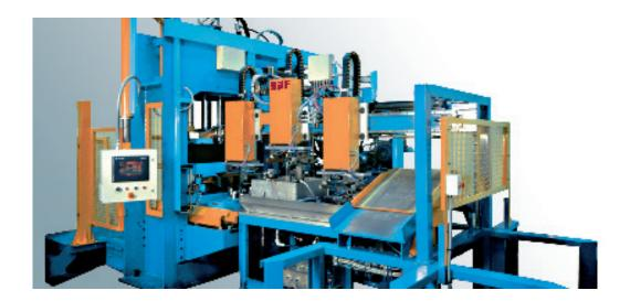
By integrating the best measuring and non-destructive test equipment, SiiF carries out the inspection operations specified by the manufacturer downstream of the finishing process.
