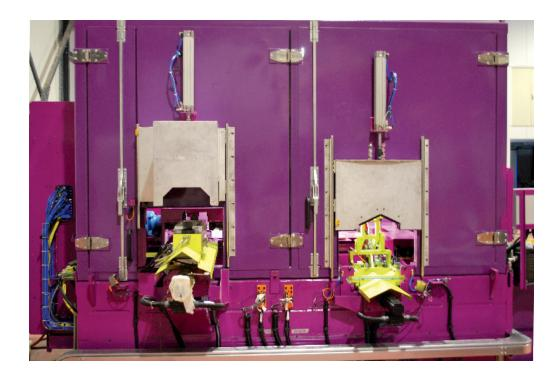
Mainly applied to cylinder heads, SiiF cubing machines ensure the dimensions of the castings prior machining.
