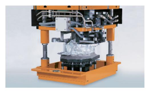
SiiF provides trimming dies for aluminum castings produced in high pressure die casting, low pressure or gravity die casting.
