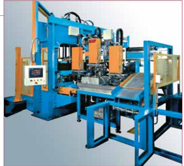
→ Trimming machine and testing line for suspension arms
