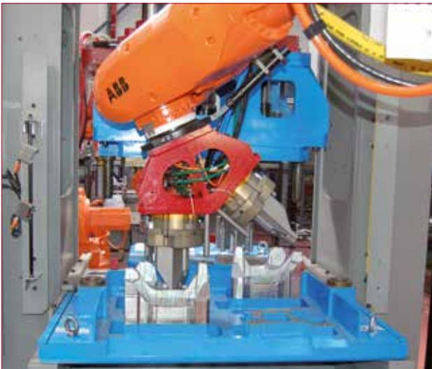
→ Robot loading of "Arcade" trimming machine
