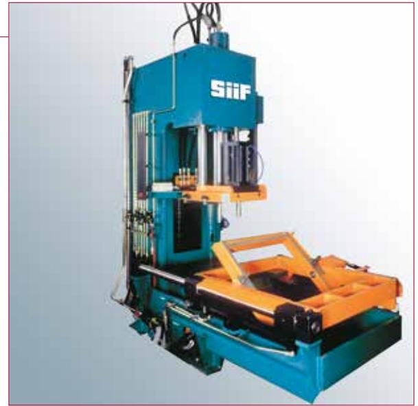
→ Trimming machine for HPDC castings with turnover shuttle for lower die cleaning
