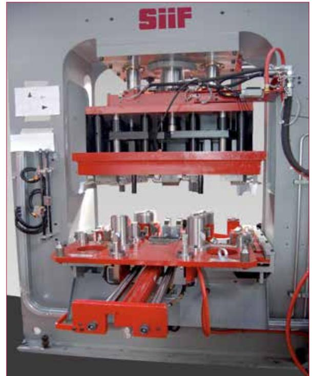
→ "Arcade" trimming machine with shuttle
