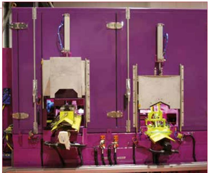
→ Cubing machine aluminum cylinder head
