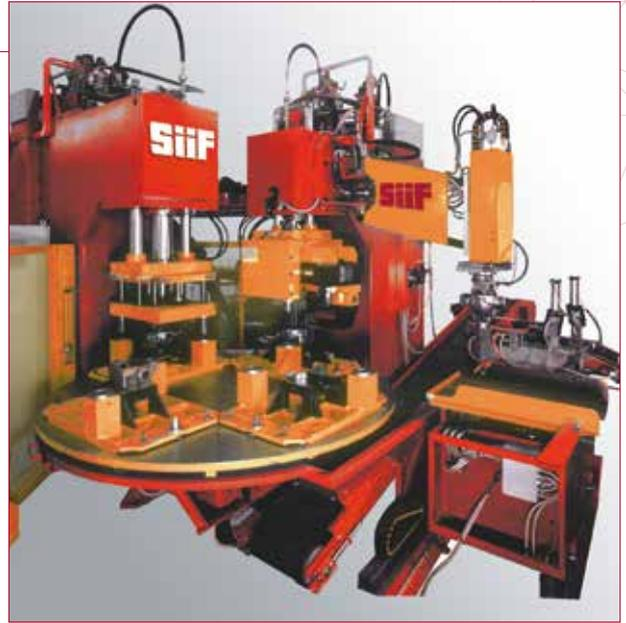
→ Four station rotary machine with differential case tooling
