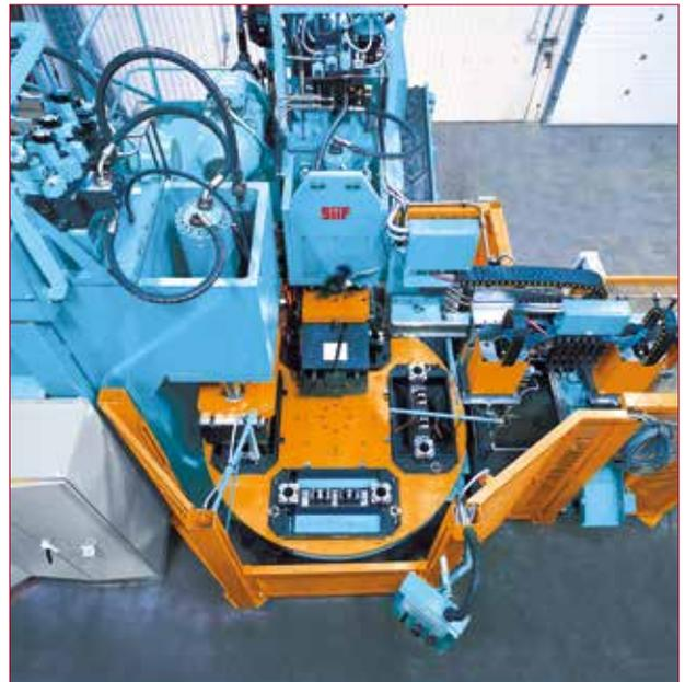
→ Four station rotary machine with brake caliper tooling
