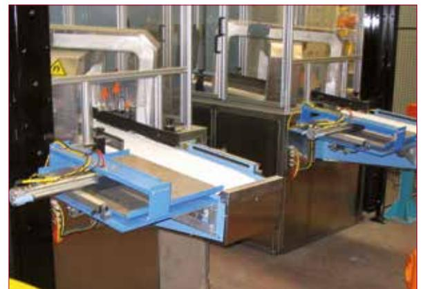
→ Tandem of 2 magnetic particle lines (800 p/h)
