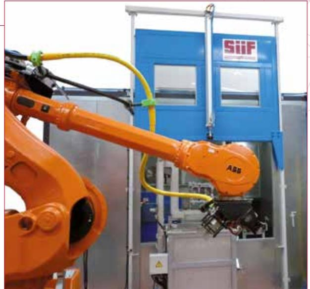
→ Robotized cell for aluminum castings
