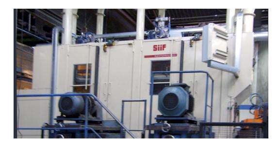
For the finishing of iron engine blocks and cylinder heads SiiF proposes 4 face grinding machines.
