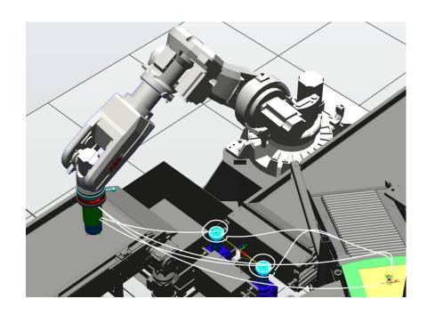
All the SiiF robotised cells can be programmed offline. These programming methods are the best way to reduce significantly the production stop when creating a new reference. Offline programming of 3D vision from the CAD piece.
