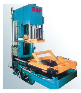
SIIF has developed a complete range of shuttle trim machines for single plane trimming. Used for trimming brake parts, knuckles, manifolds, brackets etc. either in iron or aluminum.
