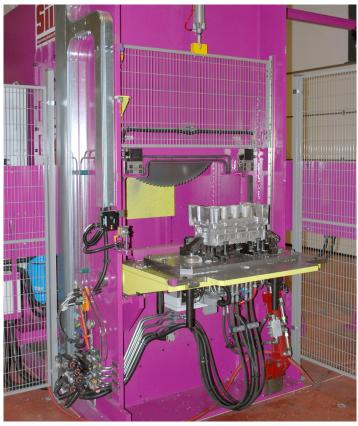
SiiF has developed a circular saw for cutting feeders from aluminium casting parts.
