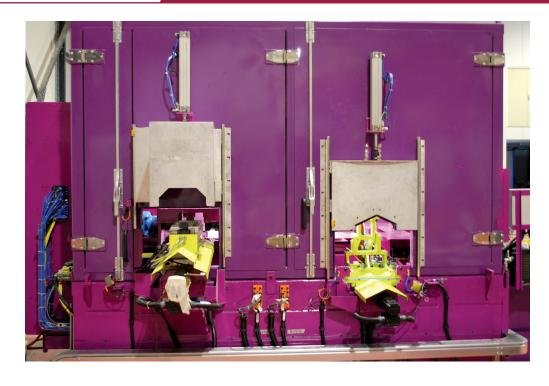
Mainly applied to cylinder heads, SiiF cubic volume machines ensure the dimensions of the parts prior to machining.
