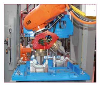
→ Robot loading of "Arcade" trimming machine
