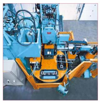
→ Four station rotary machine with brake caliper tooling
