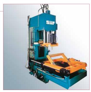
→ Trimming machine for HPDC castings with turnover shuttle for lower die cleaning
