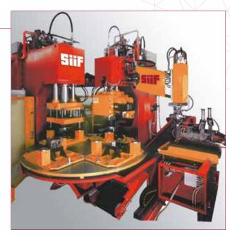
$\rightarrow$  Four station rotary machine with differential case tooling
