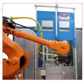
→ Robotized cell for aluminum castings
