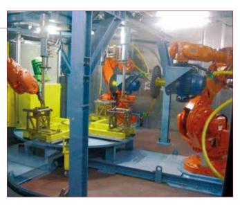
→ Robotic cell for iron parts (145 shaker arms /h, 280 differential cases /h)
