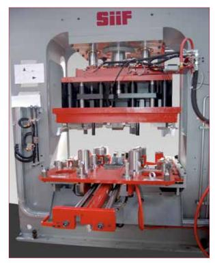
→ "Arcade" trimming machine with shuttle
