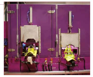
→ Cubing machine aluminum cylinder head
