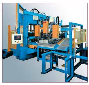
→ Trimming machine and testing line for suspension arms
