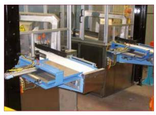
→ Tandem of 2 magnetic particle lines (800 p/h)
