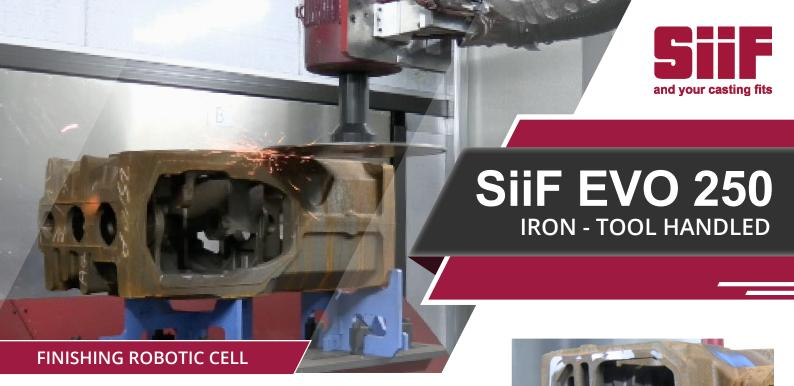
Max. casting dimensions 1100 mm x 700 mm x 650 mm Max. casting weight 250 kg
